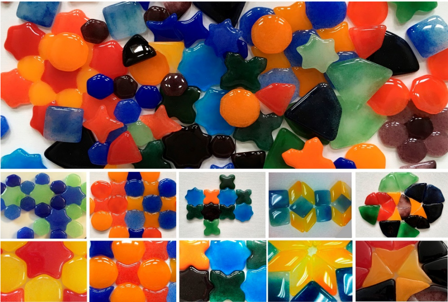
Figure 8. The final casted glass results from the five experiments Source: (Ajlouni 2018).
