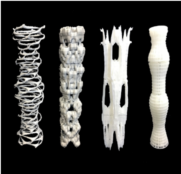
Figure 1: 3D printed structures generated using cellular automata algorithms based on studies of growth of cellular structures (Project credits: Jennifer McElroy).
