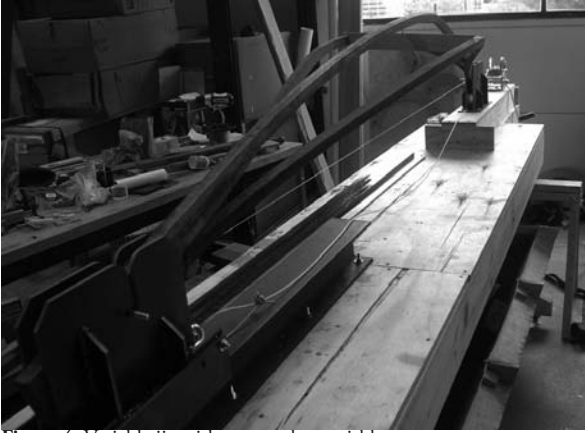
Figure 4: Variable jig with a steam bent wishbone
