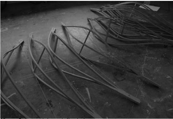
Figure 5: Formed, braced ribs drying
