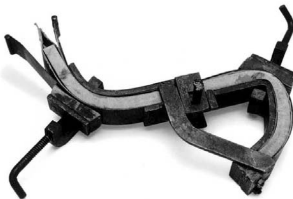
Figure 11: Early Thonet cast iron mold. Source: (Vongesack, 1997)
