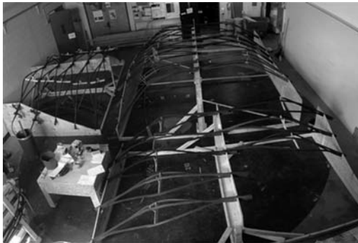
Figure 14: CNC cut fabrication forms
