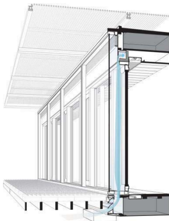
Figure 10 Section through the south façade from BIM model Figure 6 Façade elevation
