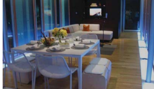
Figure 9 LED lights arranged in strips embedded in the floor vary in color and intensity. All light coves and luminaires change colors from a "warm" 2700 k to neutral 4000 k and daylight 5400 k. This allows different lighting actions in different areas, taking care of physiological and psychological needs. For example: Bedroom lighting is activated when the alarm clock sounds.
